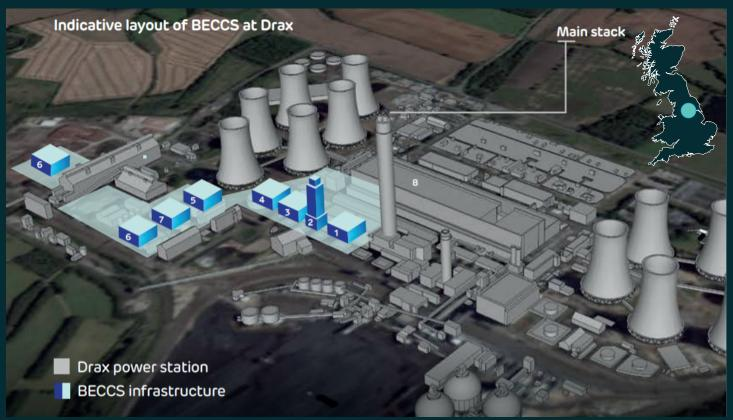
1. Flue gas pre-treatment 2. Absorber 3. Solvent heat exchangers 4. Solvent regeneration 5. Solvent storage 6. Compression and processing 7. Waste water treatment 8. Steam supply from exsiting boiler
